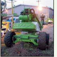
The **HR18** offers exceptional rough terrain performance due to its increased wheel size and ground clearance. Add to this a class leading working envelope and spacious 300kg capacity platform and the **HR18** stands out as one of the most robust and versatile work platforms available.
